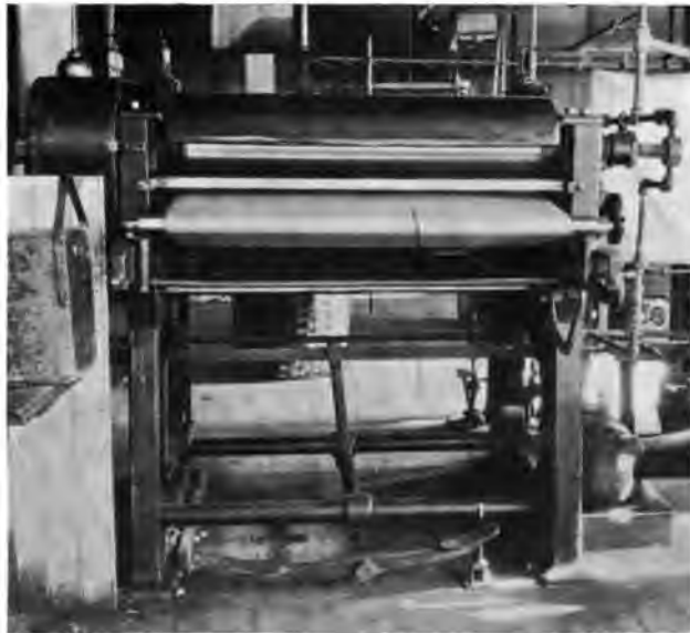
Fig. 3. Collar and Cuff Ironer with Fixed Guard for Rolls, Gear Guards, Heat Deflector and Treadle Latch.
